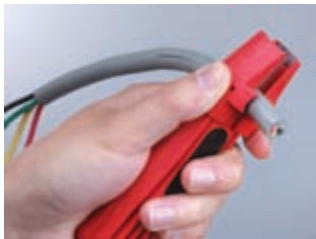
纵向剥割带护套电源线 Longitudinally stripping and cutting power cord with sheath
