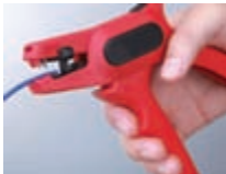
调节剥电源线尺寸 Adjust the dimension of stripping power cord
