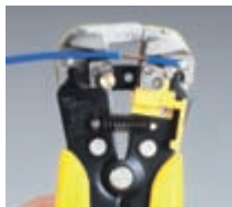
剥线 10-24 AWG (0.2-6.0mm 2 ) Wire stripping 10-24 AWG (0.2-6.0mm 2 )
