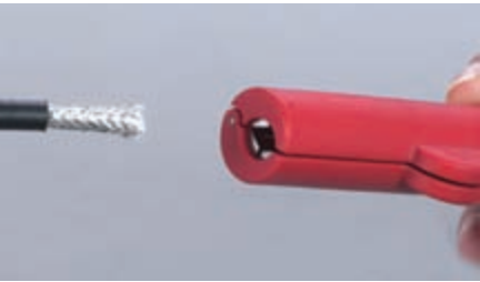
直径 5.0~15.0mm 的 UTP+STP 数据电缆的剥皮 The stripping of UTP+STP data cable in the diameter of 5.0~15.0mm
